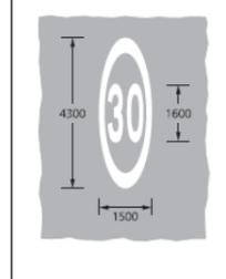
Roseworthy from Camborne. **40** MPH Repeater roundel must be used in conjunction with upright repeater. The smaller repeater roundel size being used as < 40mph. Min 150mm spacing from double white lines to avoid visual bleeding of lining.
