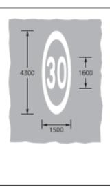
**40MPH** Roseworthy from Connor Downs. 40mph repeater roundel must be used in conjunction with upright repeater. The smaller repeater roundel size being used as < 40mph. **Off set** towards the centre of the road. Min 150mm spacing from double white lines to avoid visual bleeding of lining.
