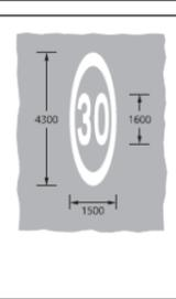
40MPH Roseworthy from Connor Downs. 40MPH Repeater roundel must be used in conjunction with upright repeater. The smaller repeater roundel size being used as < 40mph. Min 150mm spacing from double white lines to avoid visual bleeding of lining.
